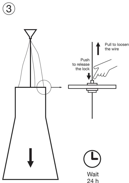
Loosen all three steel wires and let the whole weight of the lampshade rest on the power cord only.
