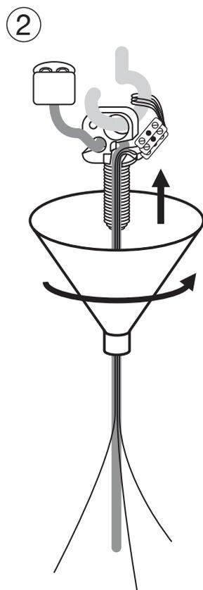
Insert the wires into the cord slot.
